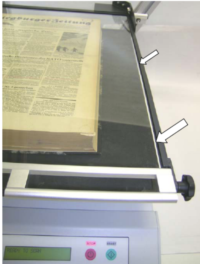
Picture 8: Horizontal alignment check
